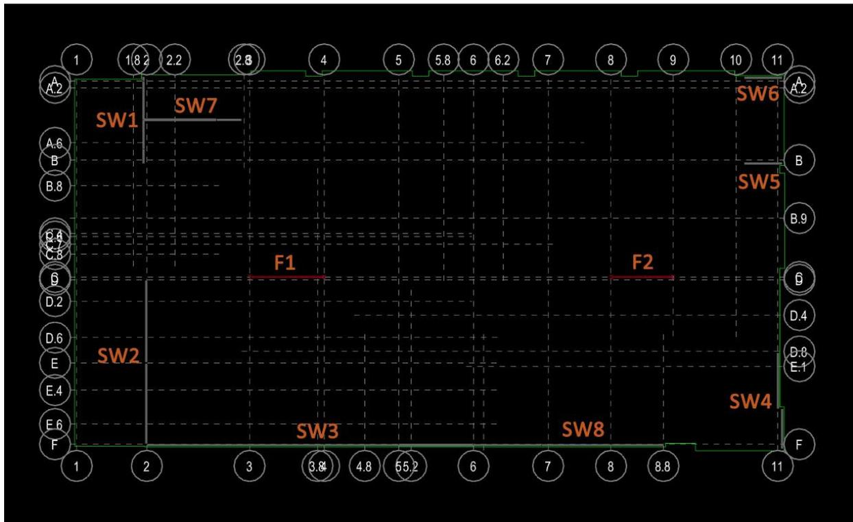
Figure 34: Floor plan displaying frame and shear wall designations.
