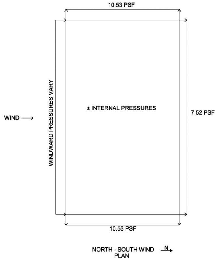
Figure 23 : Summary of pressures in the North-South direction in plan.
