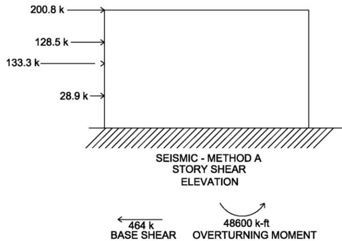
Figure 29 : Summary of forces due to seismic loads.
