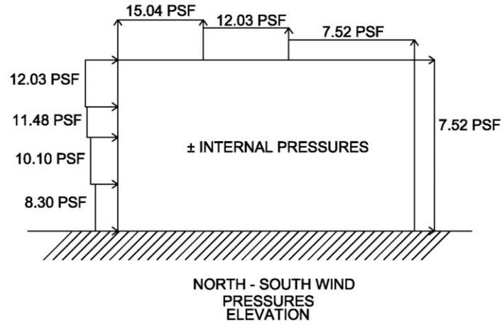
Figure 22 : Summary of forces in the North-South direction in elevation.
