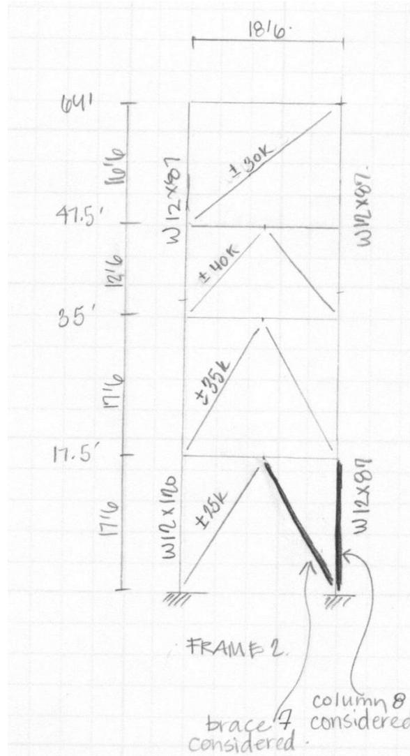
Figure 48: Elevation of braced frame 2, with verified members highlighted on right.
