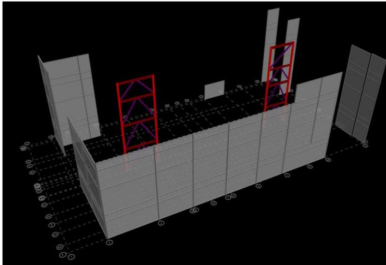
**Figure 33:** RAM model showing lateral system without diaphragms.
