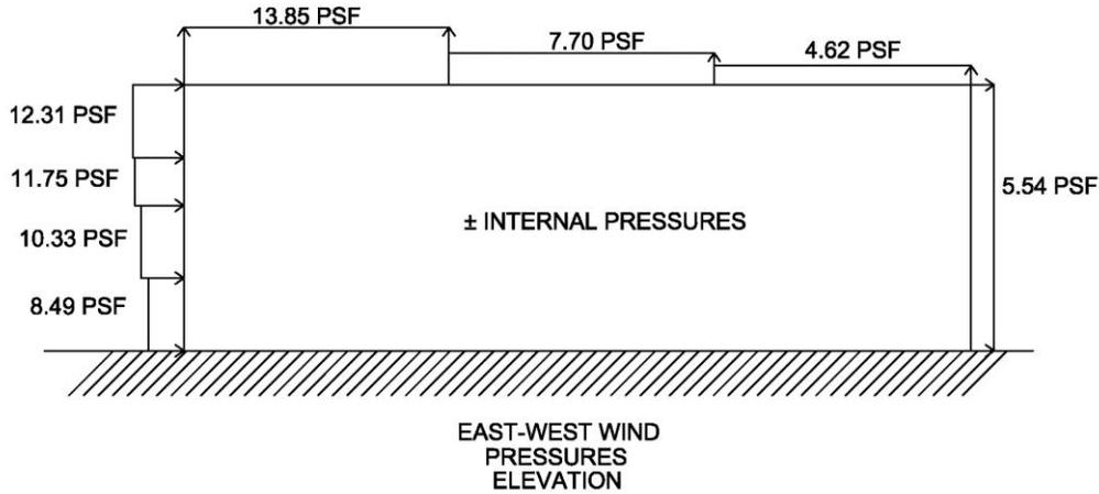
Figure 17 : Summary of East-West wind pressures in elevation.
