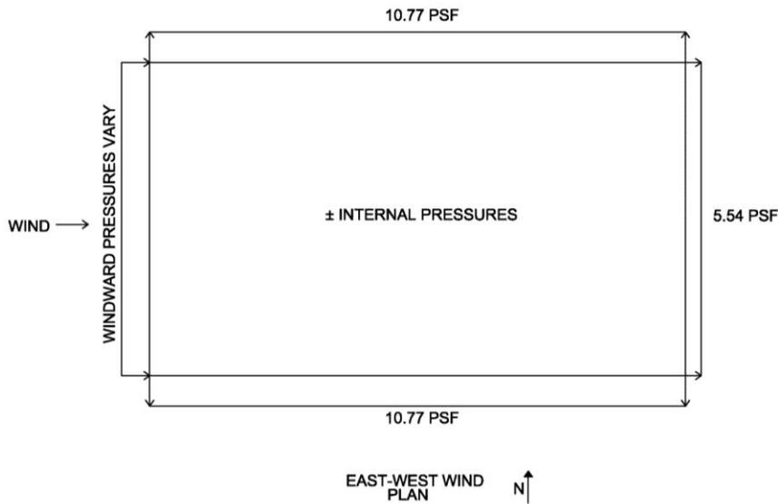
Figure 18 : Summary of East-West wind pressures in plan.
