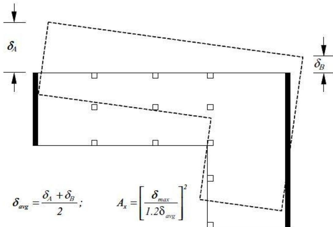
FIGURE 12.8-1 TORSIONAL AMPLIFICATION FACTOR,  $A_x$
