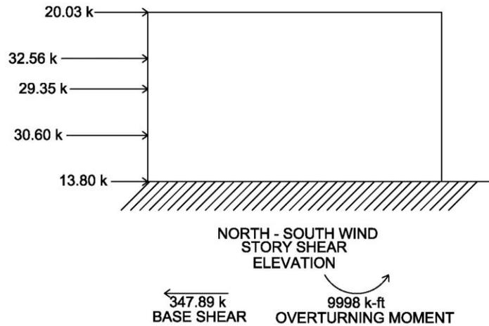
Figure 25 : Summary of final forces in North-South direction in elevation.
