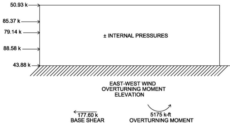
Figure 20 : Summary of final forces in East-West direction in elevation.
